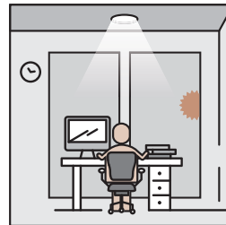
The luminaire is switched on at maximum or dimmed to maintain the lux level. The luminaire is dimmed according to the level of available daylight.
