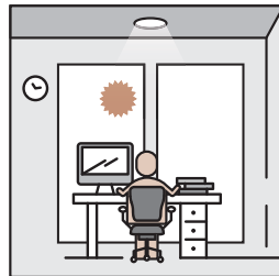
The luminaire is switched on at maximum or dimmed to maintain the lux level. The luminaire is dimmed according to the level of available daylight.
