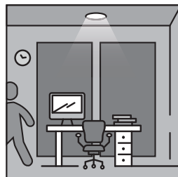
The light is dimmed during the standby period and remains at the selected minimum dimming level.
