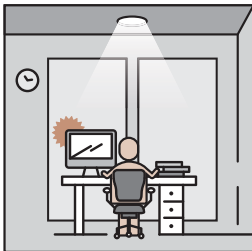
The luminaire is switched on at maximum or dimmed to maintain the lux level. The luminaire is dimmed according to the level of available daylight.
